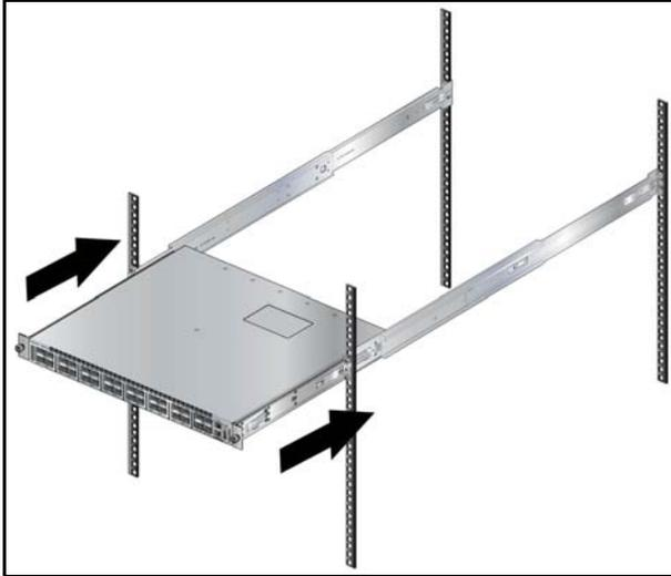
**Figure 12: Inserting the Switch onto the Rails**
