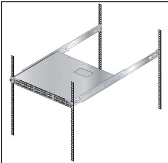
**Figure 13: Attaching the Switch to the Rack Posts**
