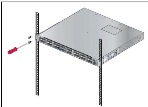
**Figure 5: Inserting the Switch into the Rack**
