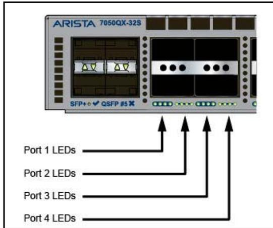
**Figure 18: Port LEDs**
