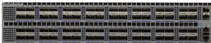
Arista 7260CX-64: 64 x 40/100GbE QSFP100ports, 2 SFP+ ports
