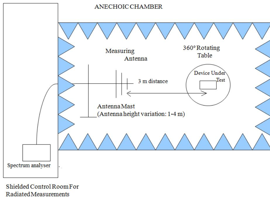
Radiated measurements setup  $f > 1$  GHz:
