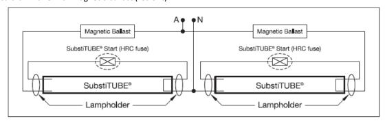
**NOTE:** If a luminaire contains a power factor correction capacitor, it is recommended to remove it from the circuit to maintain power factor >0.9. This should only be carried out by a licensed electrician.
