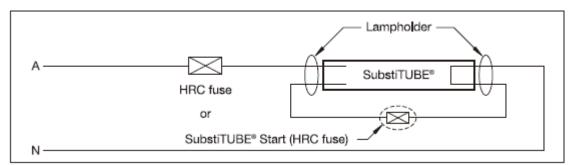
Wiring configuration for new or modified luminaires with double circuit:
