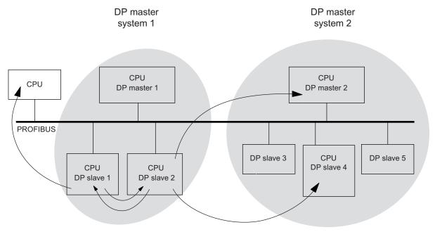
Figure 8-1 Direct data exchange via DP CPUs
