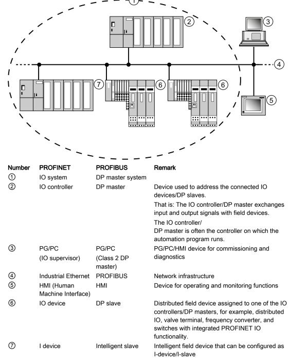
Figure 4-3 PROFINET and PROFIBUS devices
