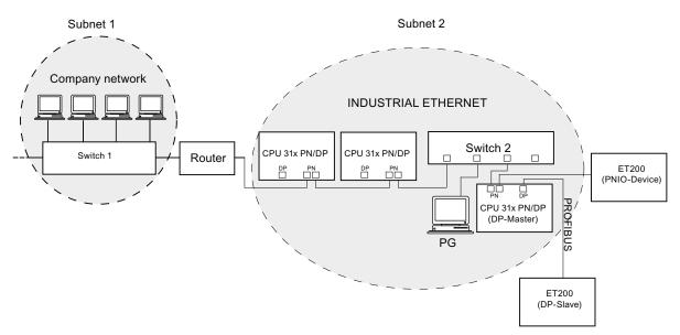
Figure 4-7 Example of a PROFINET subnet
