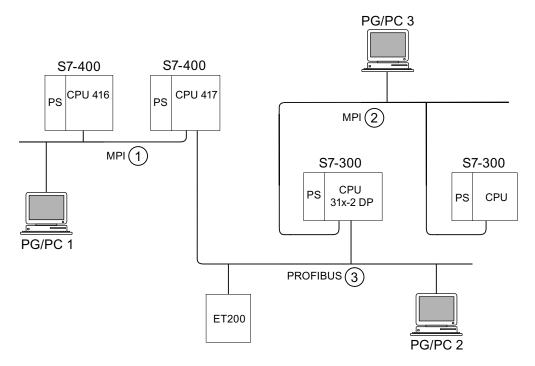
Figure 4-8 Access to remote networks
