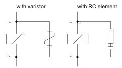
Properties of a protective circuit with varistor:
