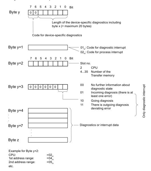
Figure 10-7 Device-specific diagnostics
