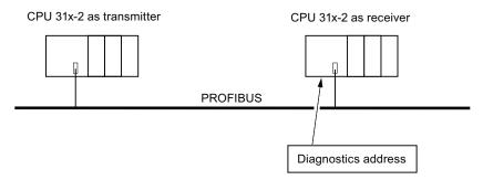
Figure 10-3 PROFIBUS DP diagnostics address
