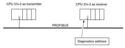
Figure 10-2 PROFIBUS DP diagnostics address
