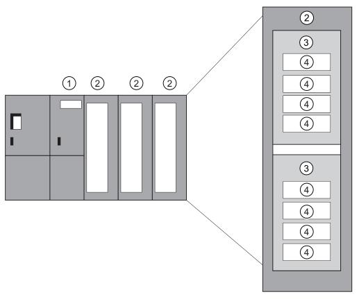
Figure 4-4 Module, Submodule, Slot, and Channel
