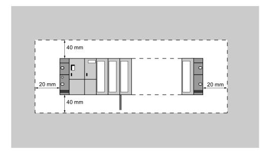
5.3 Installing modules on the mounting rail
