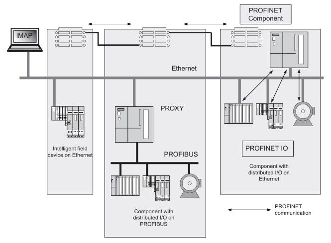
Figure 4-5 PROFINET CBA - modular concept
