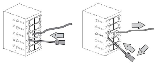
Figure 6-2 Disconnecting the wiring of a 40-pin Fast Connect connector
