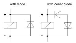
Diode/Zener diode circuits have the following characteristics:
