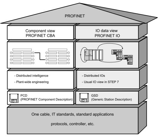
Figure 4-6 Extent of PROFINET CBA and PROFINET IO
