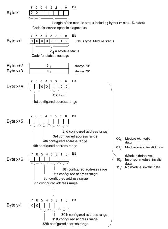
Figure 10-6 Structure of the module status for CPU 31xC
