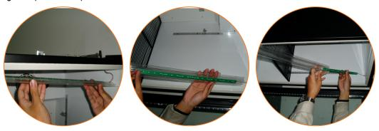
3 Disconnect the LED light strip at the Quick Disconnect.
