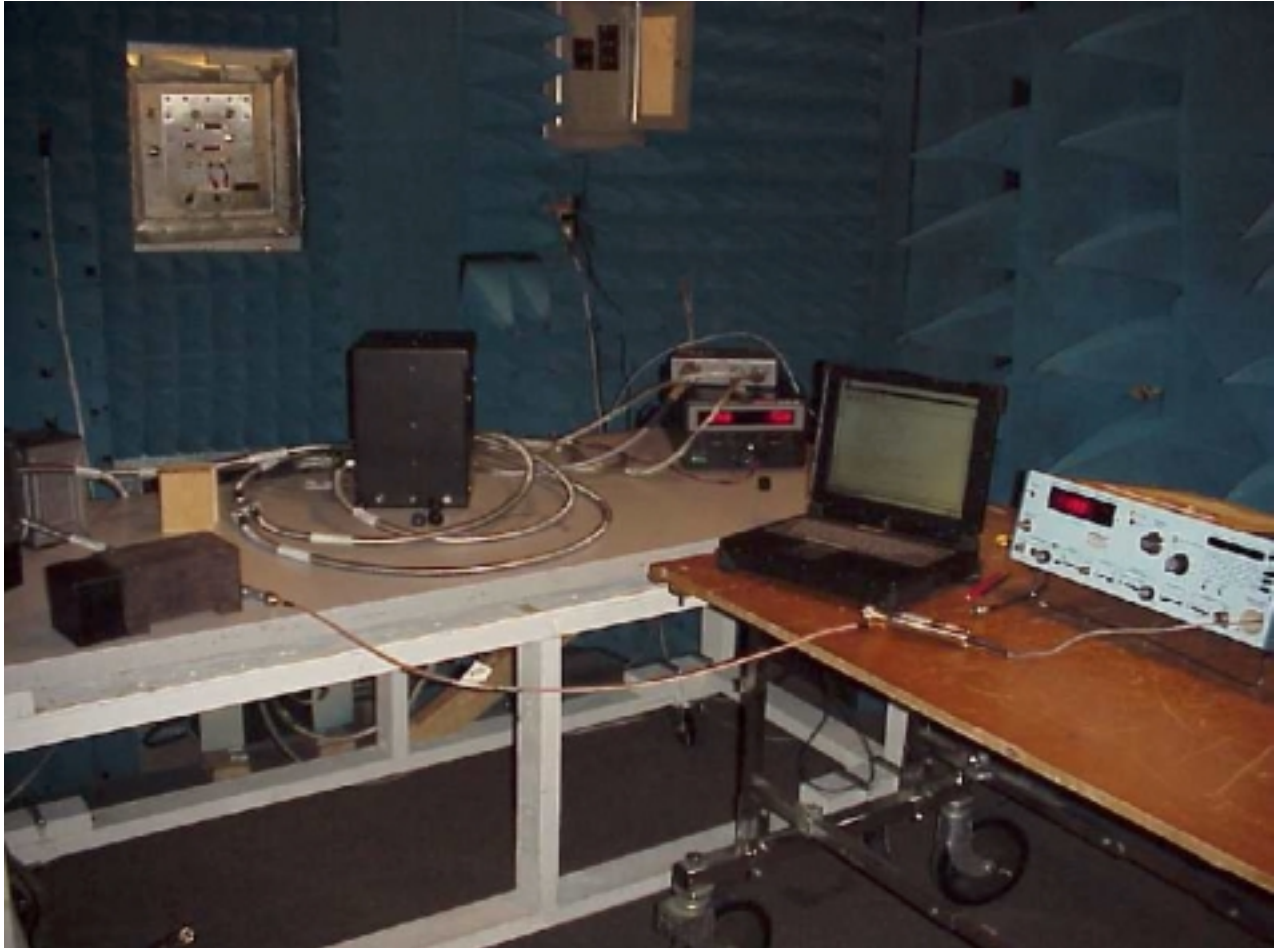
Photo H.2 LCM RF chamber test setup at Rubicom Systems, Inc.
