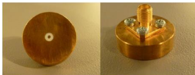
Figure 1 – MVG LIMESAR Dielectric Probe
