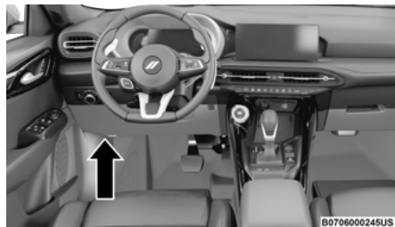
Interior Fuse Box Location
