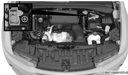
Positive (+) Battery Post
