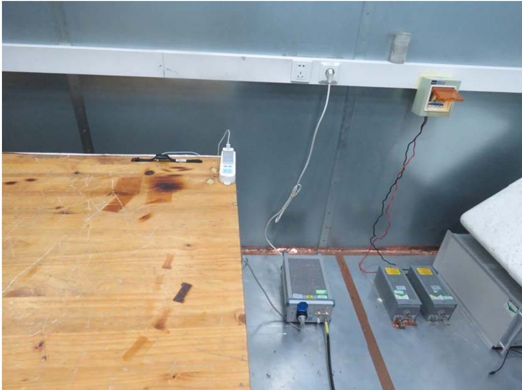
Picture 2 Conducted Emission Test Setup
