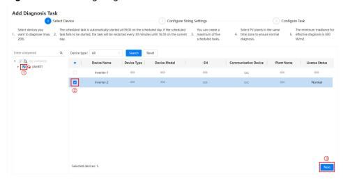
Figure 4-7 Selecting target devices
