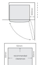
When positioned in a corner, the clearance must be at least 300mm on the hinge side to allow the door to open smoothly so that bins and shelves can be removed easily.
