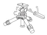
Loosen the Pan & Tilt Handle to tilting, the Panning Lock Knob to panning and move the camera into the desired shooting position. Turn the Handle and the Knob clockwise to lock the camera in position.
