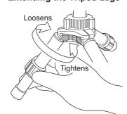
To extend any leg, turn the Leg Lock Nut one helf turn counterclockwise.
