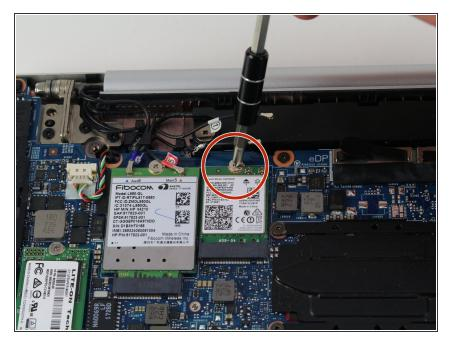
• Remove the single 2mm screw that is holding the WiFi card in place using the Phillips #1 screwdriver.
