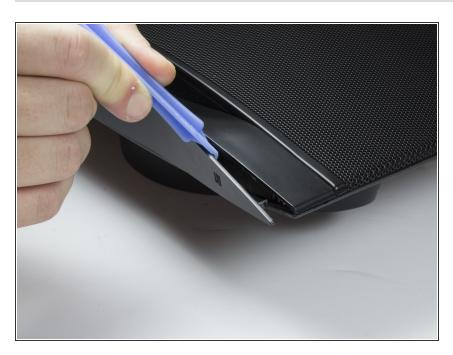
Flip speaker around and use a plastic opening tool to remove the top panel from the speaker.
