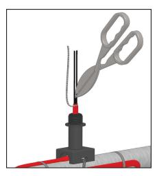
Use tin snips or similar tool to cut excess material from between the buss wires.
