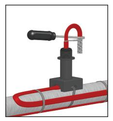
**4.** While bending the heating cable, work the cable through the braid opening. Pull the braid tight.
