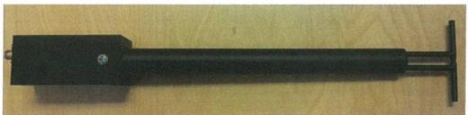
Figure 1 - MVG COMOSAR Validation Dipole
