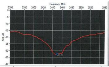
Frequency (MHz) Return Loss (dB) Requirement (dB) Impedance 2450 -32.61 $52.3 \Omega + 0.3 j\Omega$
