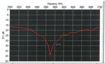
Return Loss (dB) Requirement (dB) Frequency (MHz) Impedance 2600 -32.7349.9 Ω + 2.3 jΩ
