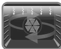
**Double Grill and Fan Function:** The oven's thermostat and warning lights will switch on, and the grill, upper heating elements and fan will
