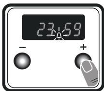
2. Select the desired time period using the “+” and “-” keys while
