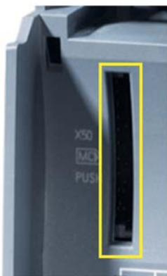
Figure 3-1 Slot for the SD card (yellow frame)
