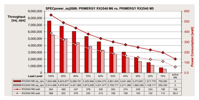
The total average throughput of the PRIMERGY RX2540 M6 is 43,933,444 ssj\_ops, an improvement of 71.3% over the 25,641,201 ssj\_ops of the PRIMERGY RX2540 M5.
