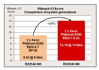
The graph on the left compares the VMmark V3 scores of the PRIMEGY RX2540 M6 and the previous generation PRIMEGY RX2540 M5.
