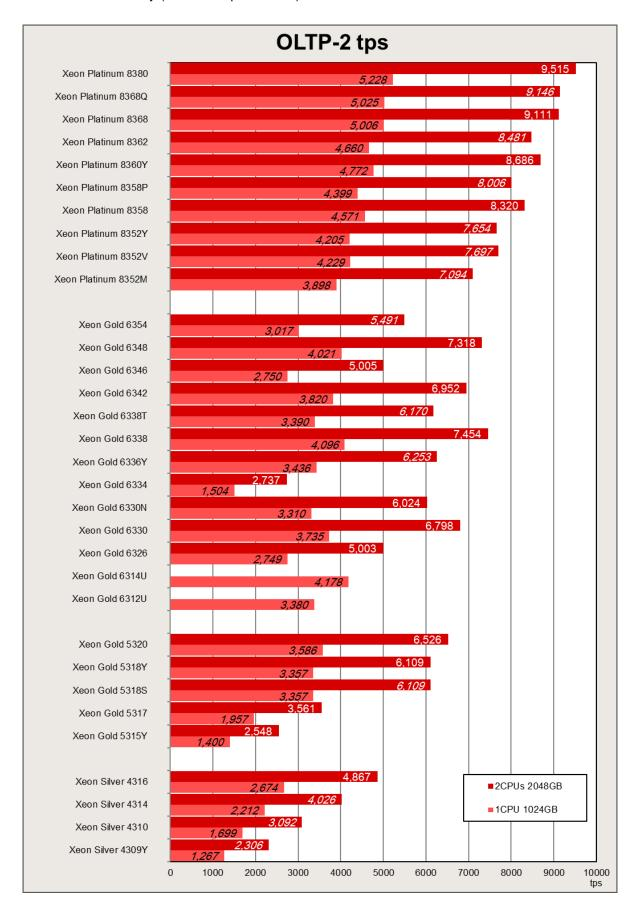
It is evident that a wide performance range is covered by the variety of released processors. If you compare the OLTP-2 value of the processor with the lowest performance (Xeon Platinum 8380) with the value of the processor with the highest performance (Xeon Sliver 4309Y) the OLTP-2 value increased by a factor of 4.
