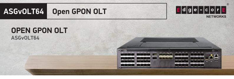
ASGvOLT64 is a 64 port GPON OLT virtual Optical Line Terminal (vOLT) with 2 fixed 40/100G QSFP28 uplink ports capable of breaking out to 4 x 25/10G, 8 fixed 10/25G SFP28. All interfaces are able to be accessed from the front panel. All 1G GPON ports are able to operate at line rate by default and support transceivers meeting 1G GPON ITU-T G.984 standards.
