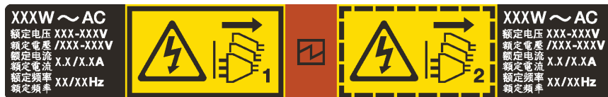
Figure 38. Hot-swap power supply label on the cover
