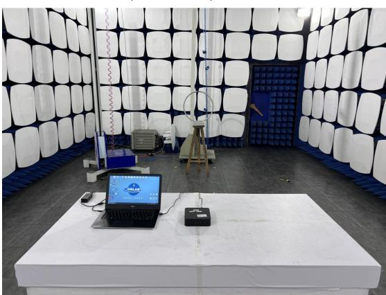
3. Radiated emission (9KHz-30MHz)
