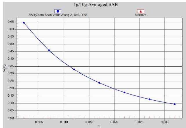
Fig.A.1- 10 Z-Scan at power reference point (W850)
