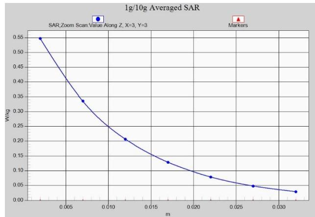
Fig.A.1- 4 Z-Scan at power reference point (PCS1900)
