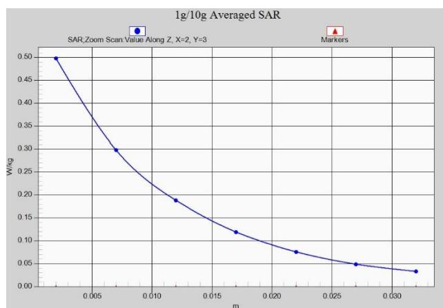
**Fig.A.1- 2 Z-Scan at power reference point (GSM850)**
