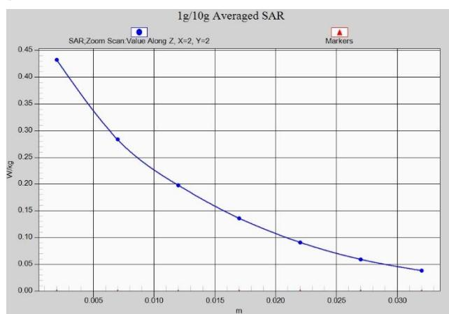
**Fig.A.1- 3 Z-Scan at power reference point (PCS1900)**
