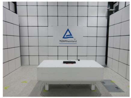
Photograph 2: Set-up for Spurious Emissions (Front View 2)
