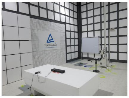
Photograph 6: Set-up for Spurious Emissions (Back View 4)
