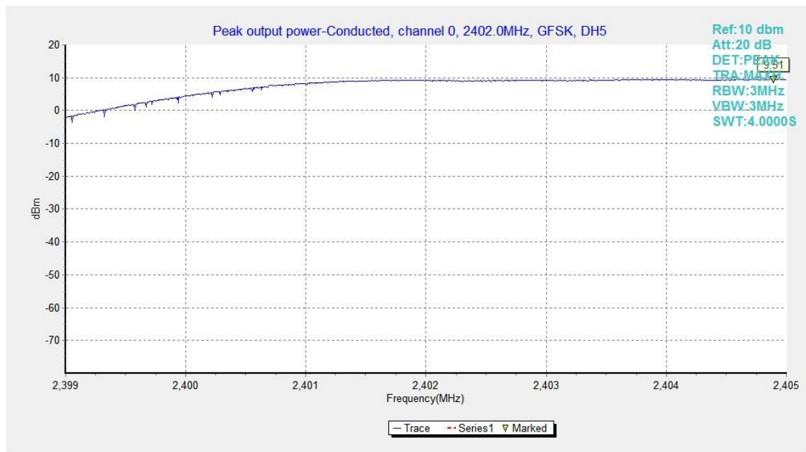
Fig.1. Peak Output Power -Conducted: GFSK, Channel 0,
