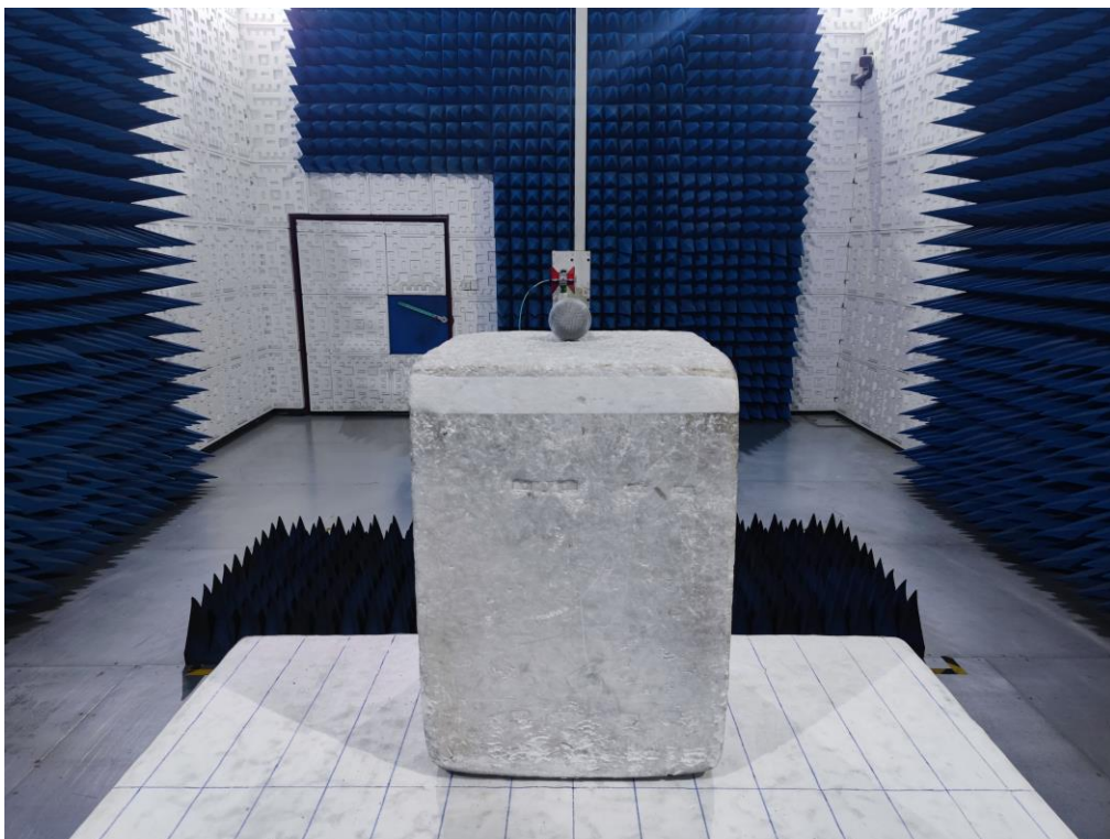
RADIATED EMISSION TEST SETUP ABOVE 1GHz
