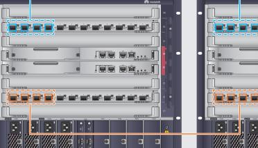
Recommended: Install LPUS symmetrically beside MPU slots. For more information. see the Hardware Installation and Component Replacement.
