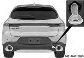
Rear Tow Eye Installed
