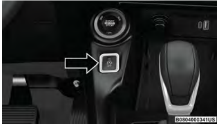
Stop/Start OFF Switch
