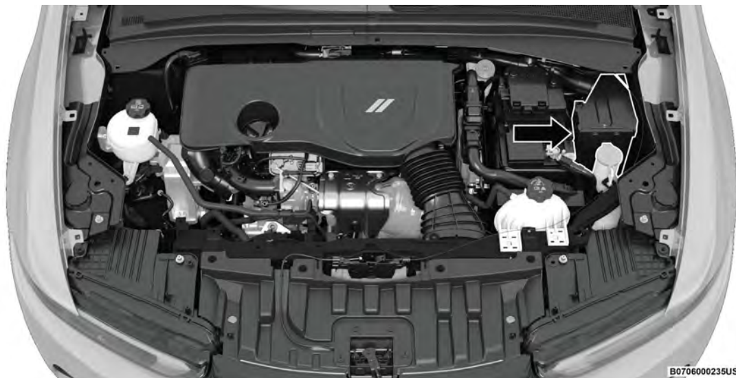
Underhood Power Distribution Location (Hybrid)
