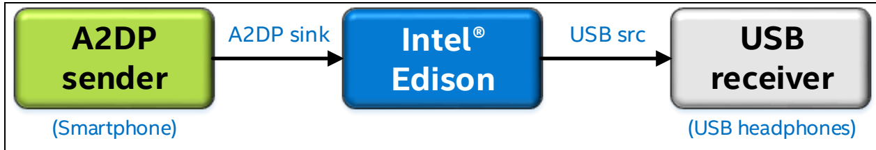
Figure 18 Bluetooth* A2DP audio source to USB sink device
