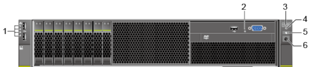
Figure 4-11 Front panel of a server with eight 2.5-inch drives
