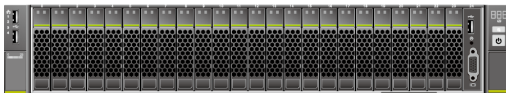
Figure 4-3 Front panel of the 2488H V5 with 24 drives
