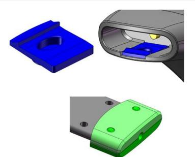
Inserting locking pin and strap
