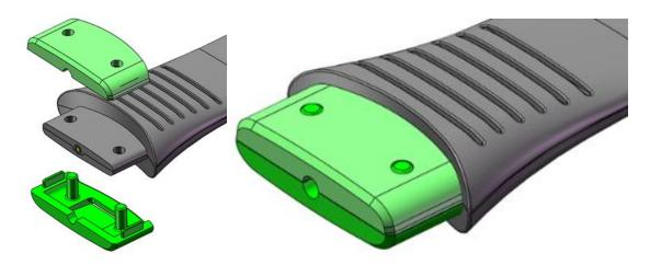
3. Fit the disposable locking clip into one end of the main body.
