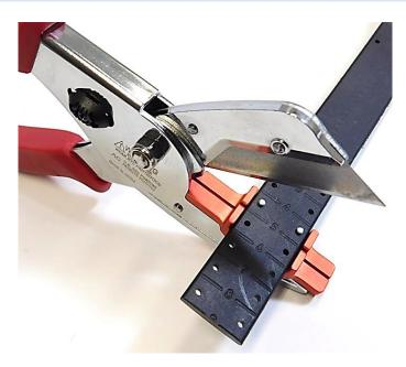
Strap cutting tool for strap length adjustment
