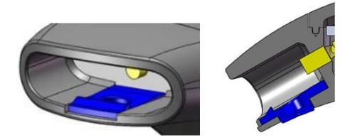
4. Fit the end of the strap into the end of the main body and push until the strap clicks in place.
