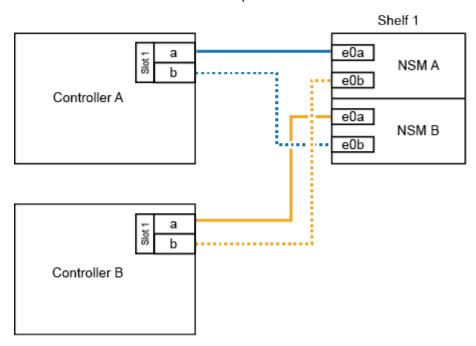
2. Verify that the hot-added shelf is cabled correctly.
