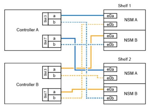
3. Verify that the hot-added shelf is cabled correctly.
