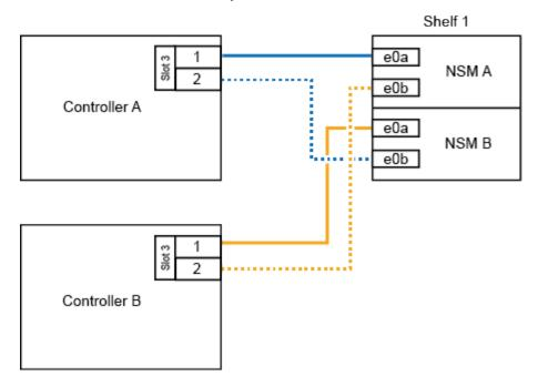
2. If you are hot-adding one or two shelves using two sets of RoCE-capable ports (two RoCE-capable I/O modules) in each controller module, complete the applicable substeps.
