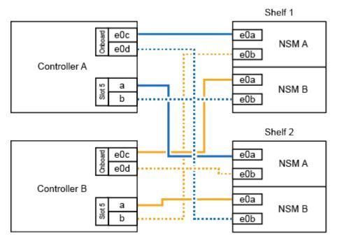
3. Verify that the hot-added shelf is cabled correctly.
