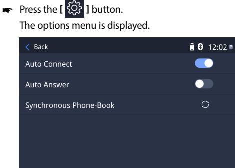
**Auto Connect** – If "Auto Connect" is activated, the device automatically connects with known Bluetooth® devices as soon as they are in range.
