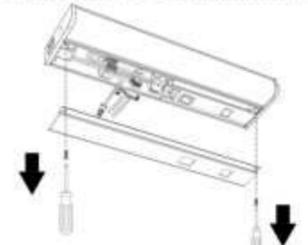
6.2 Remove the side cover and release the linking cord from the clamp inside the light compartment.
