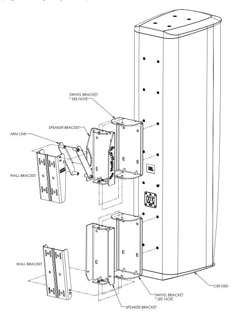
\* NOTE: Use SWIVEL BRACKETS when panning is needed for aiming speaker horizontally. When panning is not needed, leave SWIVEL BRACKETS out, and mount SPEAKER BRACKET directly to CBT 1000 cabinet. Diagram is example only. Consult IBL CBT 1000 Bracket Installation Guide for detailed installation instructions.
