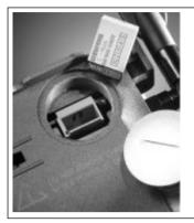
In devices with a compact housing, the C-PLUG is located behind the sealing screw on the rear of the device. To remove the sealing screw, use a coin or a wide blade screwdriver.
