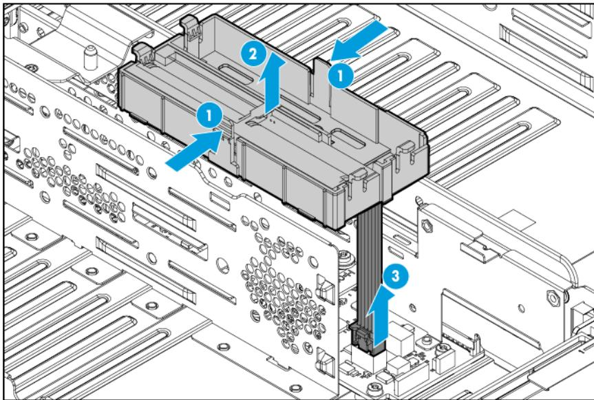
12. Remove the HP Smart Storage Battery from its holder.
