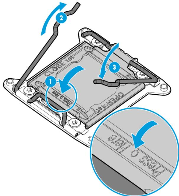
7. Install the processor socket cover on the failed system board.
