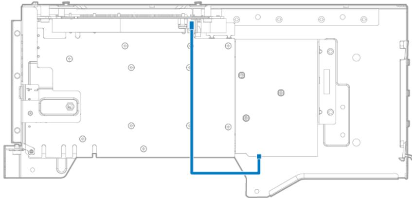
Three-slot PCI riser cage assembly and three-slot GPU-direct PCI riser cage assembly
