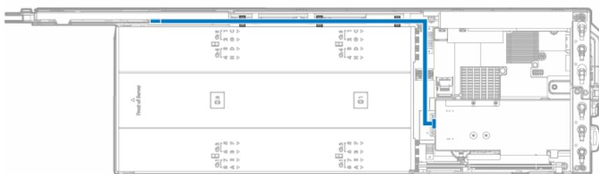
HP P840 Smart Array controller installed in a 2U node
