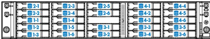
One 2U node corresponds to a maximum of eight SFF HP SmartDrives if using the HP Dynamic Smart Array B140i Controller, HP H240 Host Bus Adapter, or HP P440 Smart Array Controller.
