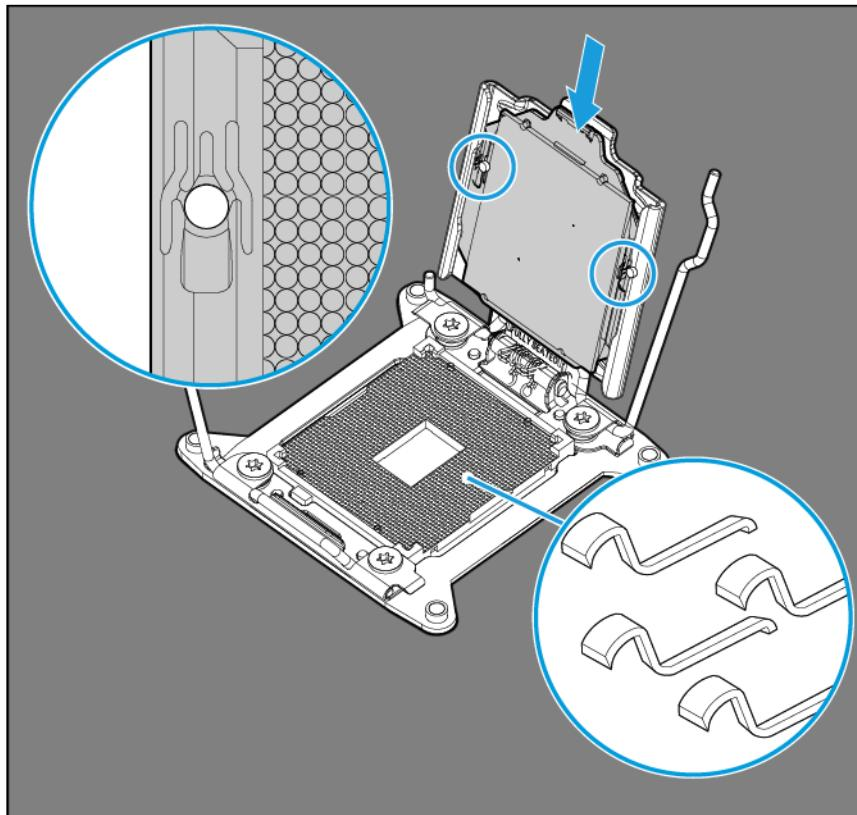
⚠ **CAUTION:** Do not press down on the processor. Pressing down on the processor may cause damage to the processor socket and the system board. Press only in the area indicated on the processor retaining bracket.
