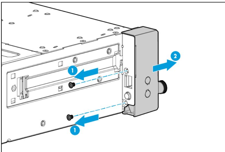
15. Disconnect the front I/O cable from the bezel ear.
