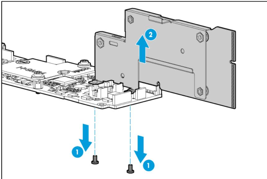
16. Remove the support bracket from the RPS link board.
