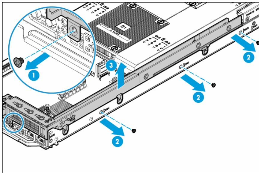
**CAUTION:** To prevent improper cooling and thermal damage, do not operate the node unless all PCI riser cages or rear I/O blanks are installed, and do not operate the node unless all PCI slots have either an expansion slot cover or an expansion board installed.
