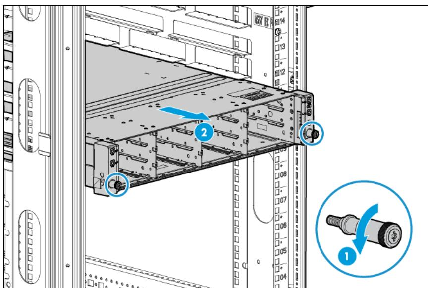
9. Remove the chassis from the rack.
