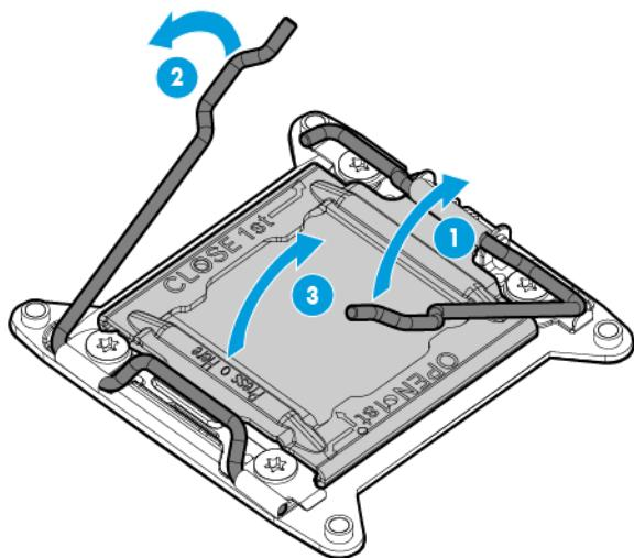
3. Remove the clear processor socket cover. Retain the processor socket cover for future use.
