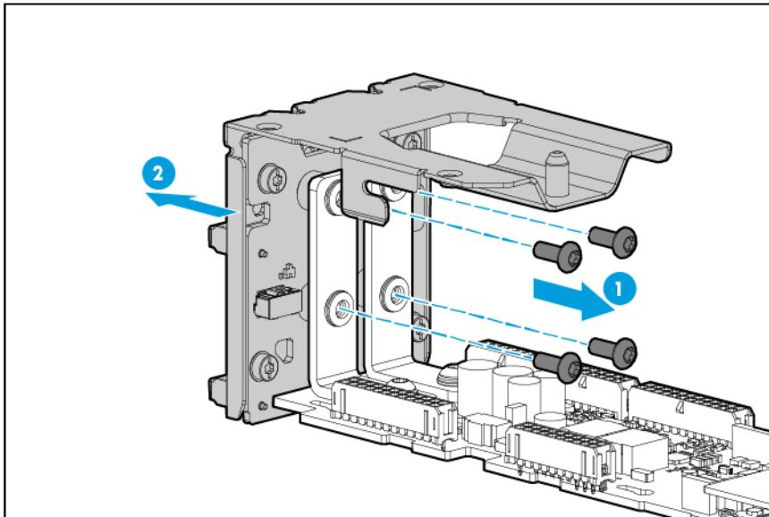
16. Using a T-15 Torx screwdriver, remove the support bracket.
