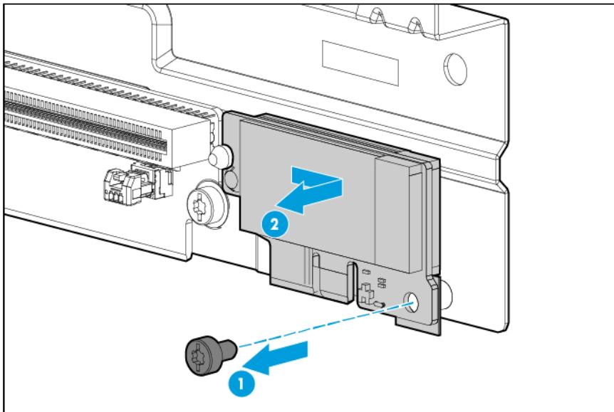
9. Loosen the T-10 screw and remove the M2. SATA SSD cards from the failed enablement board.
