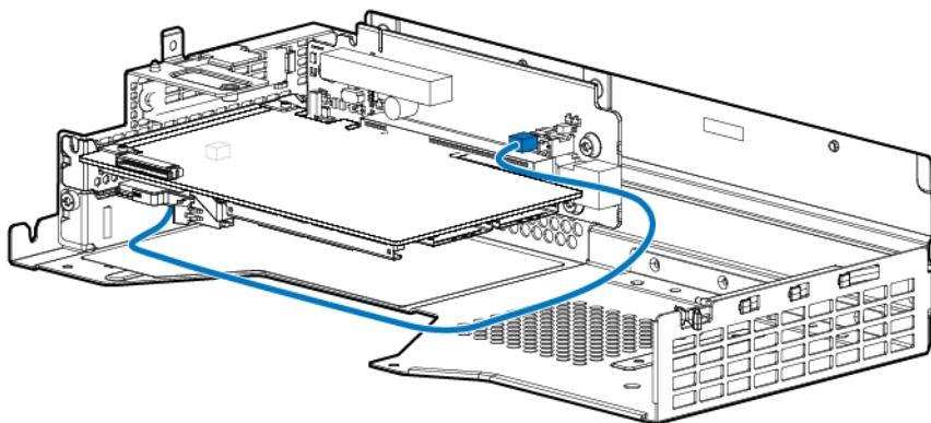
HP P840 Smart Array controller in a three-slot PCI riser cage assembly
