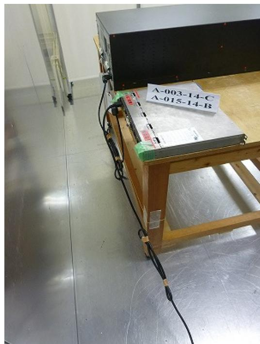
Spurious Emissions Measurement (Radiated)
