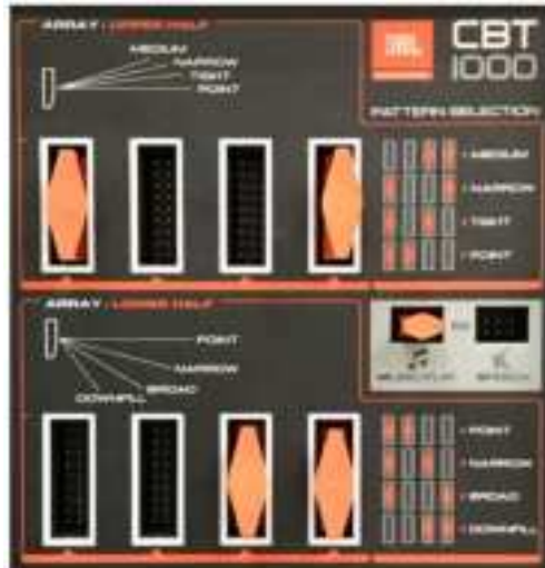
(Header position example shown above: Upper Half NARROW pattern setting; Lower Half DOWNFILL pattern setting; EQ is MUSIC/FLAT setting.)
