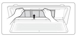
To assemble the air filter, proceed in reverse order of detaching.
