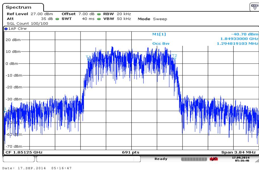
**Channel 600-Occupied Bandwidth (99% BW)**
