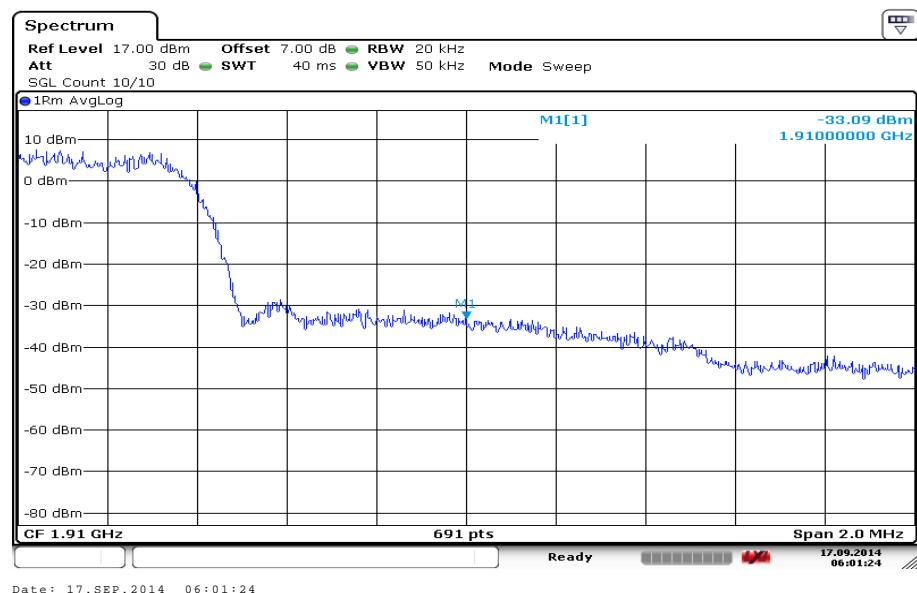
**A.6 CONDUCTED SPURIOUS EMISSION (§2.1057/§22.917/§24.238/§27.53(q))****A.6.1 Measurement Method**
