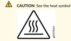
on the fan tray. The fan handle and its surfaces including the power supply handles may be hot. Wear proper protective, heat-resistant gloves while removing the fan tray.
