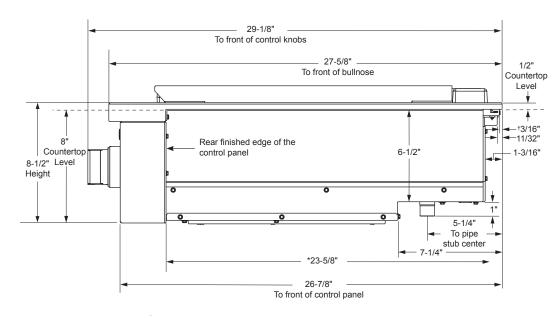
\* Minimum cabinet cutout depth from the back of the rear trim to the back finished edge of the control panel typically, the minimum cabinet depth (front to back). Maximum cabinet cutout depth is 26" minus the countertop overhang. <sup>†</sup> Include the overhang of the rear trim when countertop continues behind the product. The overhang is decorative only. The weight of the rangetop is fully supported by the side trims.
