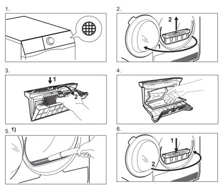
1) If necessary remove fluff from the filter socket and gasket. You can use a vacuum cleaner.
