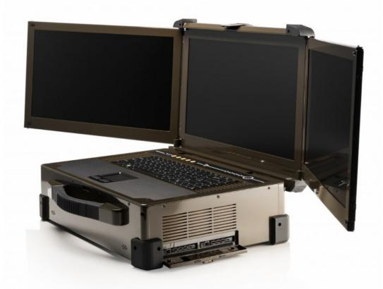
Triple display system with rugged laptop form factor and an optional battery.
