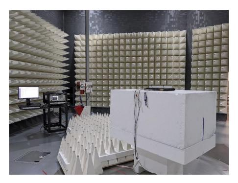
Photograph 3: Radiated Emissions 17 – 26 GHz
