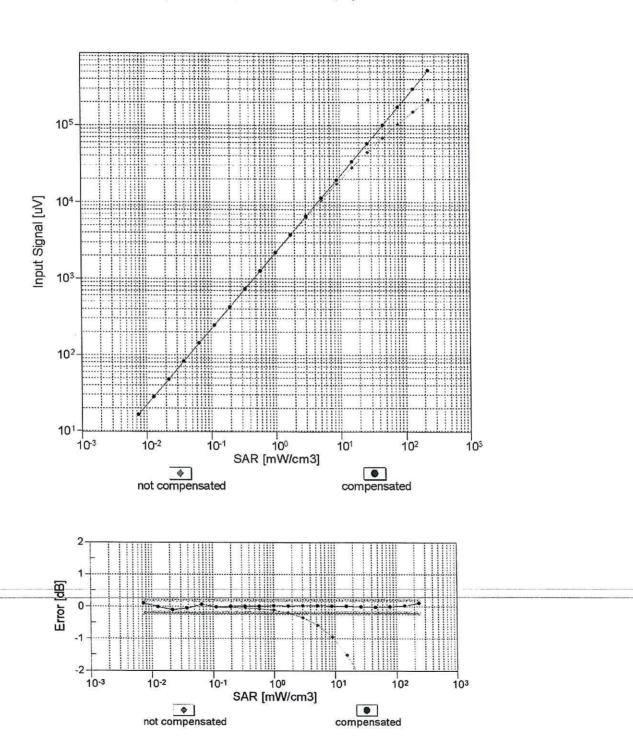
Dynamic Range f(SAR<sub>head</sub>) (TEM cell , f<sub>eval</sub>= 1900 MHz)
