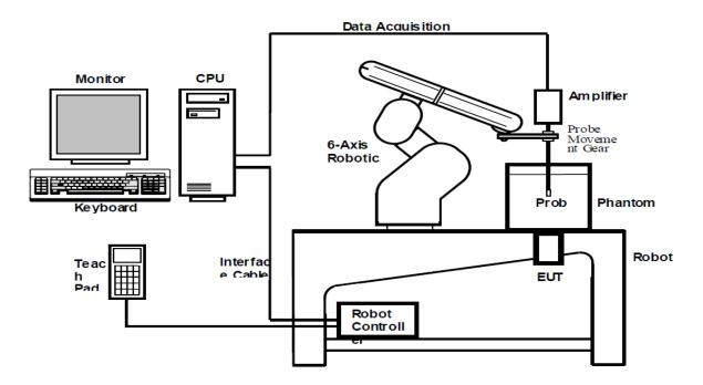
The system is remote controlled by a PC, which contains the software to control the robot and data acquisition equipment. The software also displays the data obtained from test scans by calculating the measured values into corresponding SAR values based on the currently acceptable calculation methods.
