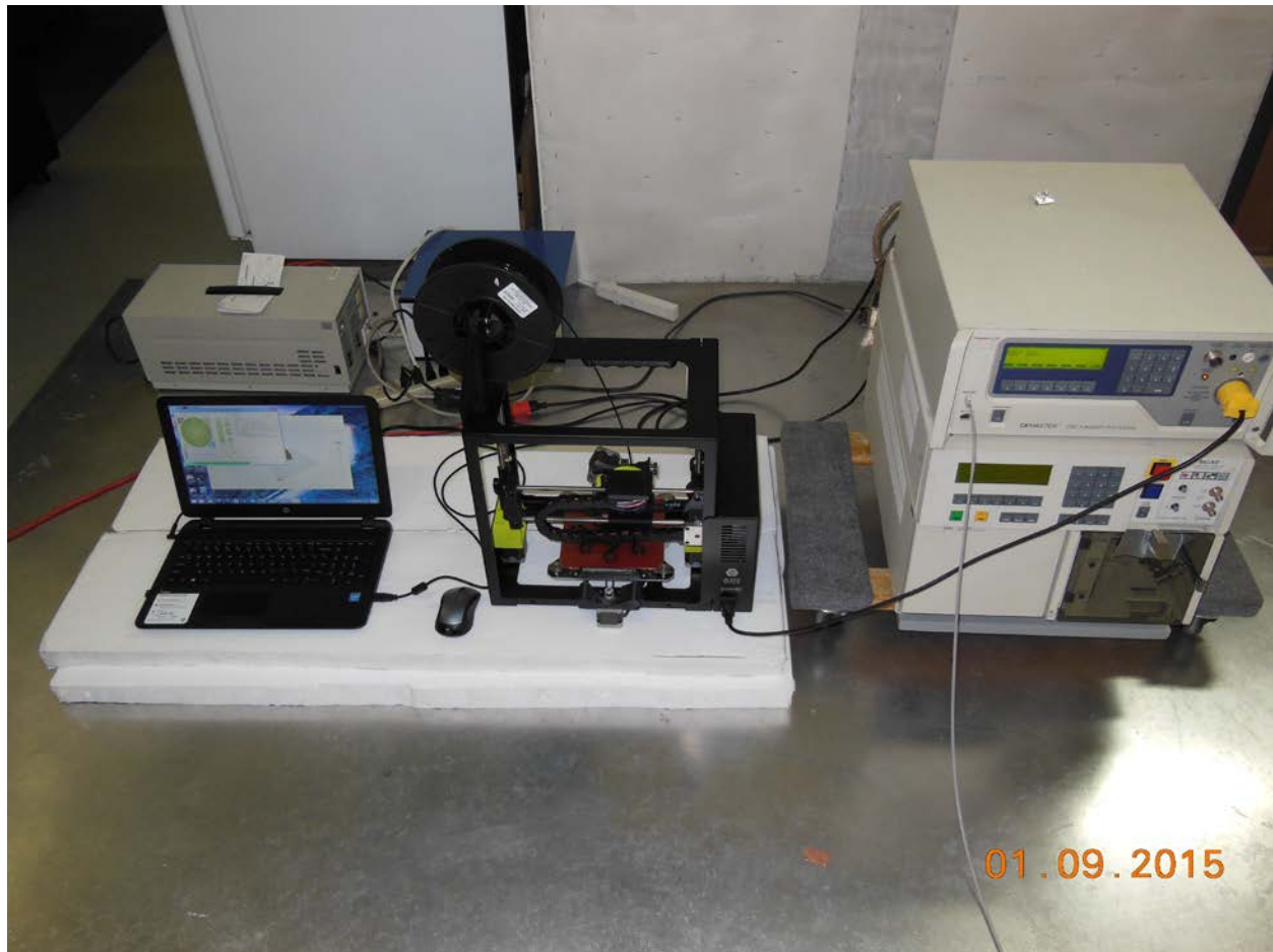
Test setup according to EN 61000-4-5, Surge
