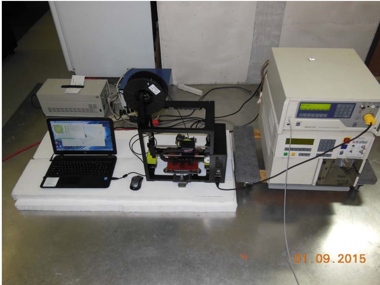
Test setup according to EN 61000-4-11
