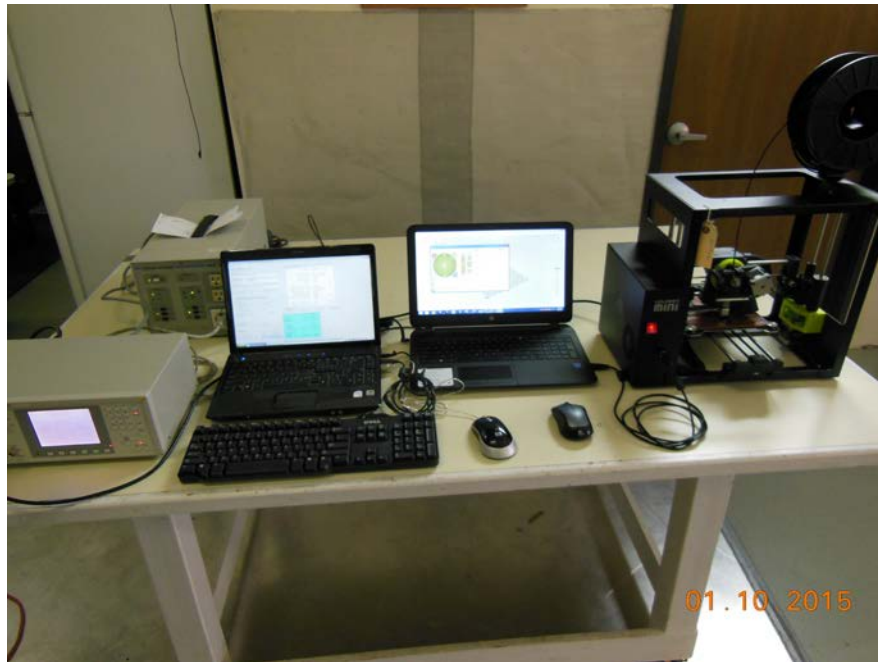
Test setup for AC power line harmonics
