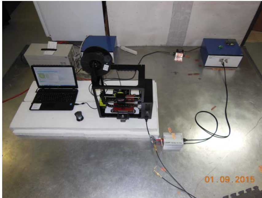
AC power line conducted immunity setup per EN 61000-4-6 The injected signal is monitored with the current clamp
