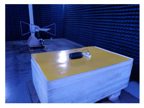
**Radiated Spurious Emissions Test View (Above 1GHz)**
