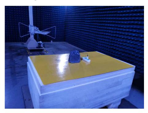
**Radiated Spurious Emissions Test View (Above 1GHz)**
